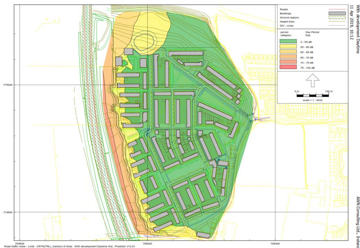
Figure 8.6 Predicted Noise Levels Across External Areas (1.5m above ground)
